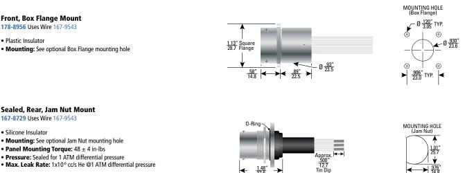
• Max. Leak Rate: 1x10<sup>-6</sup> cc/s He @1 ATM differential pressure
