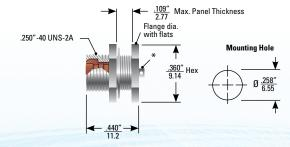
† Mates with all push-pull coupling, single-pin, PeeWee series plug or receptacle assemblies. †† Mates with all threaded coupling, single-pin, PeeWee series plug or receptacle assemblies
