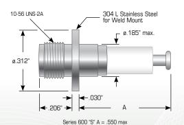
Series 600 for welded & solder flange installation A = .520
